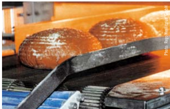
Disinfecting bread before packing
